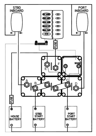
STUD A- CONNECT DIRECTLY TO THE STARTER POSITIVE OF THE STBD INBOARD.
